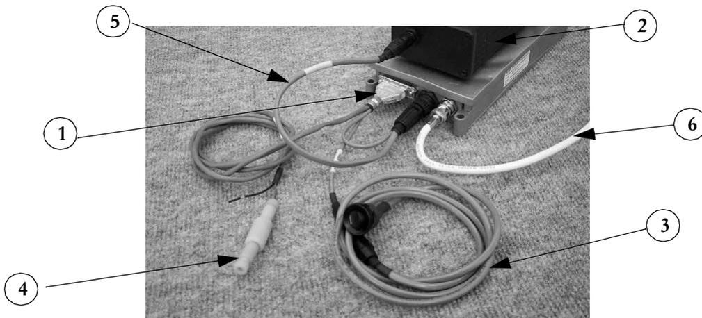
**Figure 1-5.** Overview of Main Harness Assembly, Optional Reserve Battery, Power, and VHF Antenna
