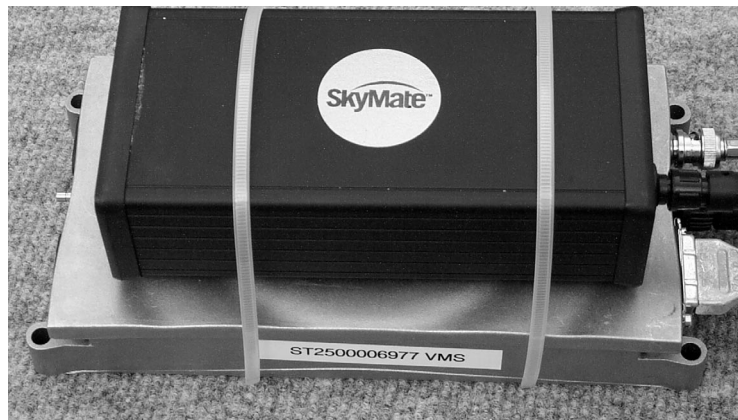
Figure 1-3. View of Installing the Optional Reserve Battery
